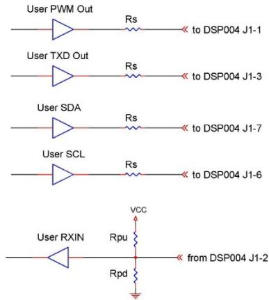
As mentioned earlier in section 1.2, a resistor of nominal 1k should be placed in series with the PWM line near the user point of signal origin, to reduce unwanted EMI from fast PWM edges, ensuring proper operation of the display.
