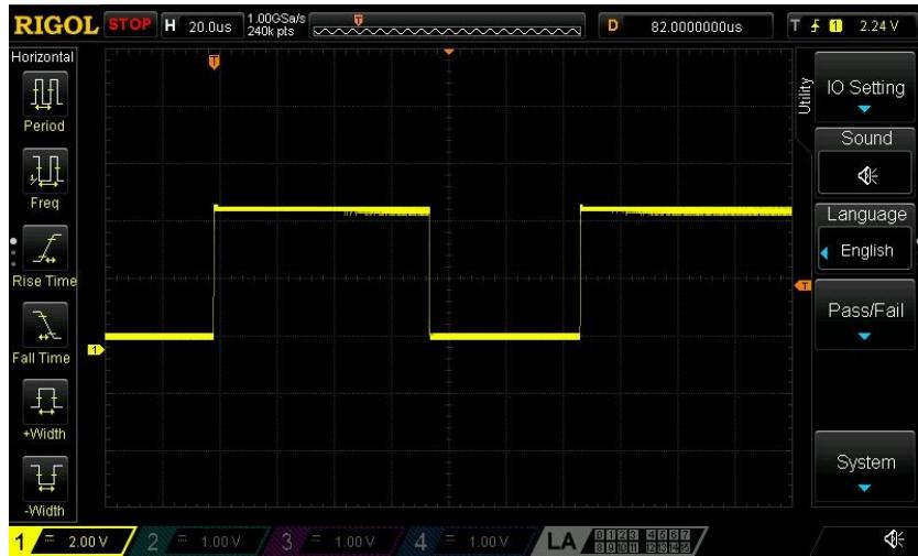
The above screenshot shows the PWM signal input, with a series 1k resistor placed near the PWM generator output. Note the generally clean waveform with minimal overshoot, with no undershoot or ringing being present.
