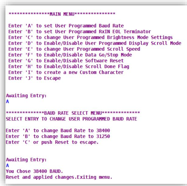
A dialog will commence asking the user to place A,B or C.The unit will operate using the selected BAUD rate when the CONFIG switch is set to the “PRGM” position. Push the MENU button again to make more selections.
