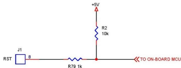
When controlling the reset pin with an MCU I/O port, ensure the port is either internally pulled up, or set to Hi-Z mode, when not active. When activating a reset function, ensure the pin is pulled low for a minimum of 10 milliseconds.
