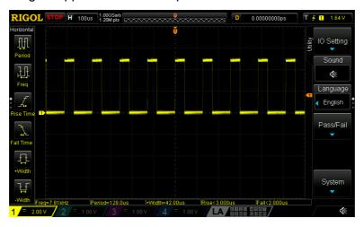
Note that frequencies other than 8kHz +/- 10% may be applied; however there is no guarantee that any such frequencies will not create interference artifacts due to the display multiplex characteristics.
