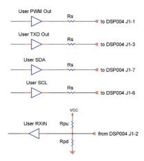
The values for Rs, Rpu and Rpd depend on the type of transmission medium and connectors used. Rs typically can have a value of 50 to 220 ohms.
